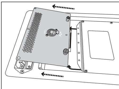
4. Slide the SL-Dante-SPK option card into the slot and line up the screw holes.
