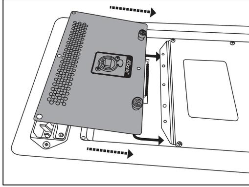
5. Push the SL-Dante-SPK option card until it locks into the internal connector and tighten the thumbscrews.
