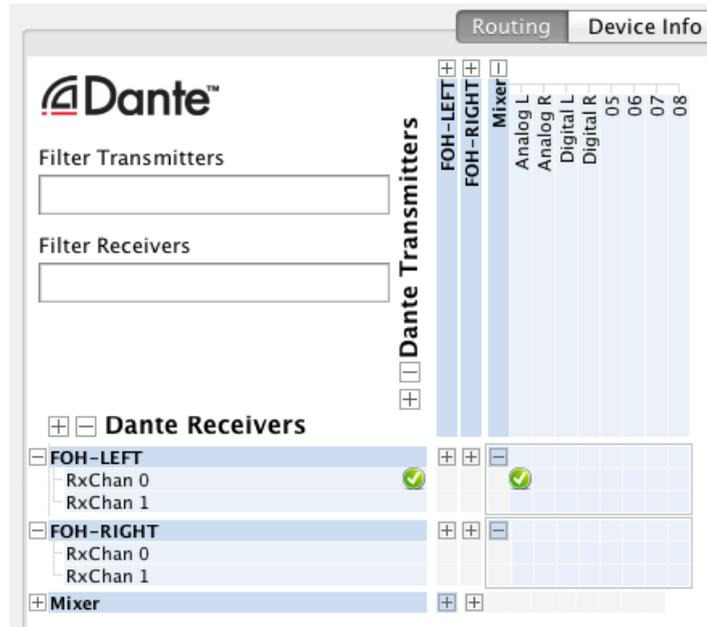
3. Continue patching Transmit channels from your mixer to the rest of the loudspeakers on your network.
