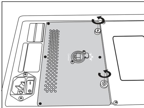
3. Gently pull the SL-Control-SPK card straight out and then slide down to remove it.
