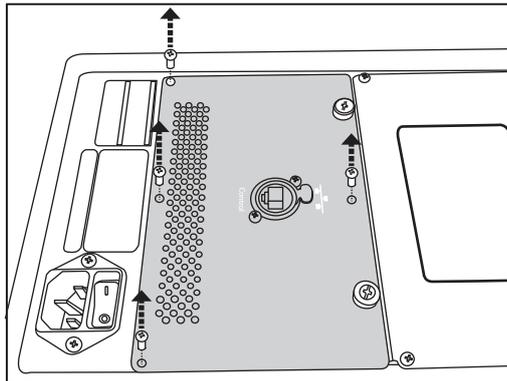
2. Loosen the two thumbscrews at the top of the SL-Control-SPK option card.
