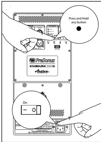
11. Power on your StudioLive AI loudspeaker while holding down any button on its back panel.
