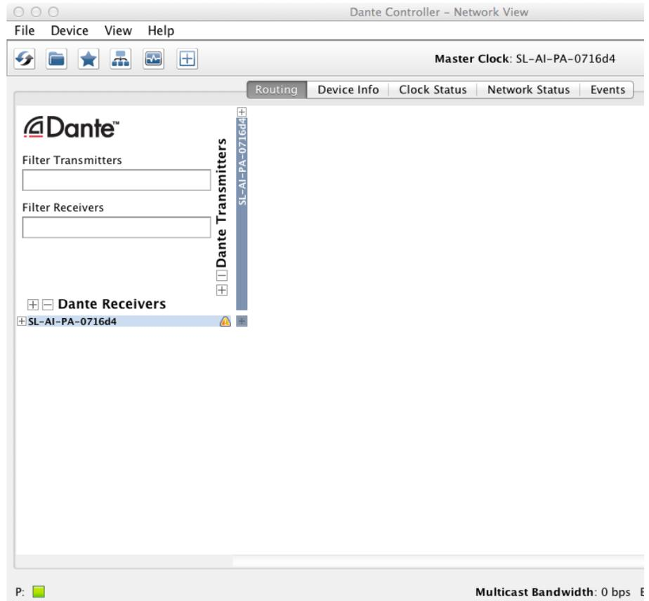
4. Open the Device view by double-clicking on the speaker name or by selecting Device>Device View.
