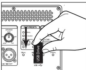
10. Connect the USB thumb drive to the USB connection on your StudioLive AI loudspeaker.
